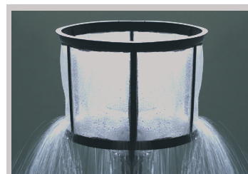
Shower head is built into the main strainer basket to easily put wearable powders into suspension
